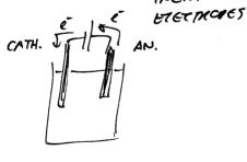
CATH  $K_{eq}^{\dagger} + e^{-} \rightarrow K_{eq}$   $\times$   $2H_{2}O + 2e^{-} \rightarrow H_{2} + 2OH^{-}\sqrt{}$ AN  $2J^{-} \rightarrow J_{2} + 2e^{-}\sqrt{}$   $2H_{2}O \rightarrow O_{2} + 4H^{4} + 4e^{-}\sqrt{}$
